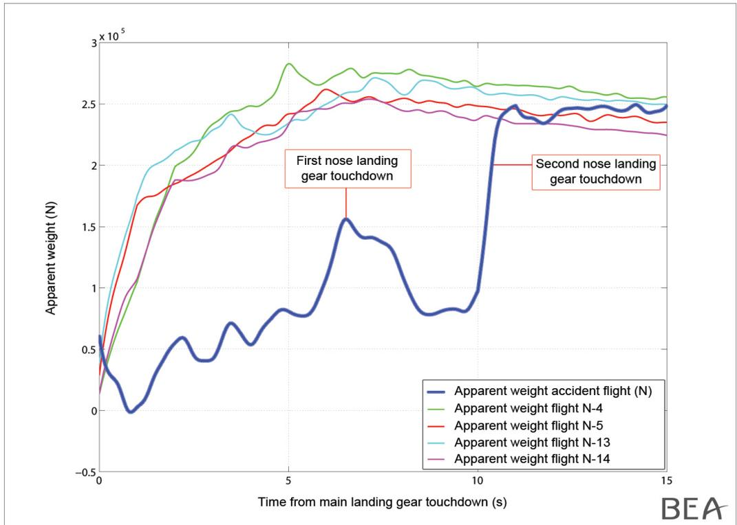
Figure 17: comparison of the apparent weight
