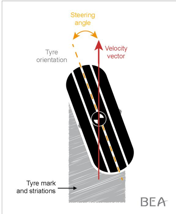
Figure 23: orientation of striations during tests, schematic diagram
