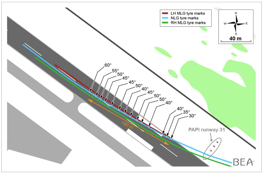
Figure 14: striation angle values along the nose gear marks
