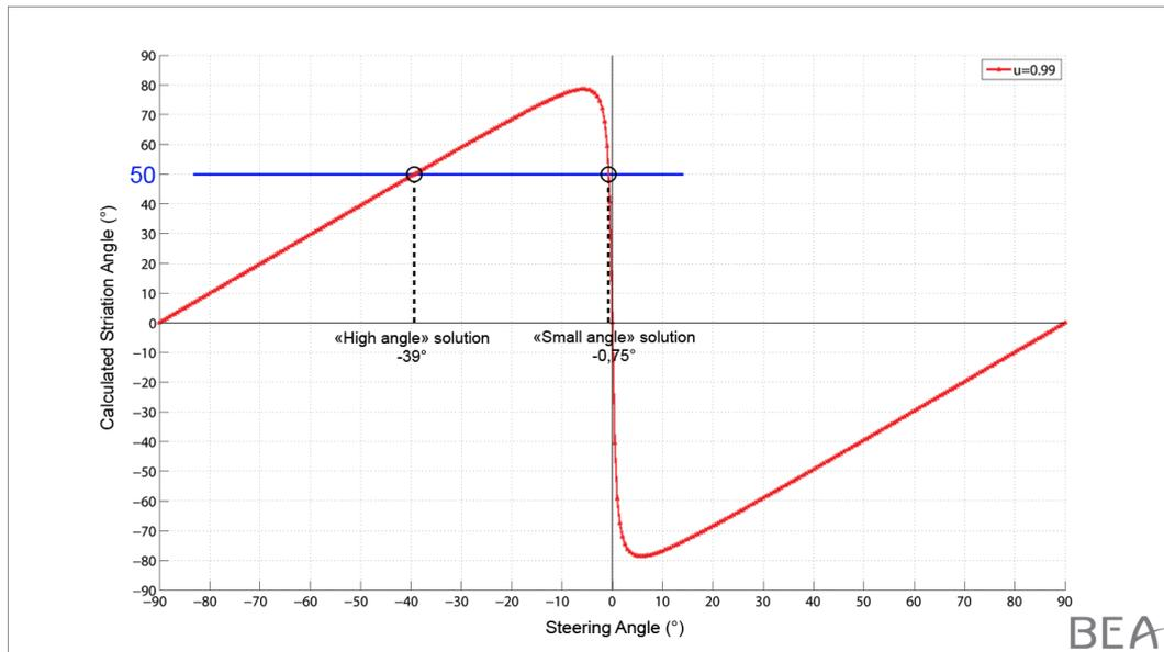
Figure 25: example of a striation angle value in relation to wheel orientation, for wheel rotation speeds close to their theoretical maximum value ( $u = 0.99$ )
