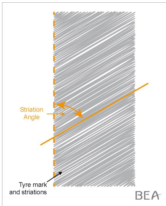
Figure 2: convention for measuring the striation angle
