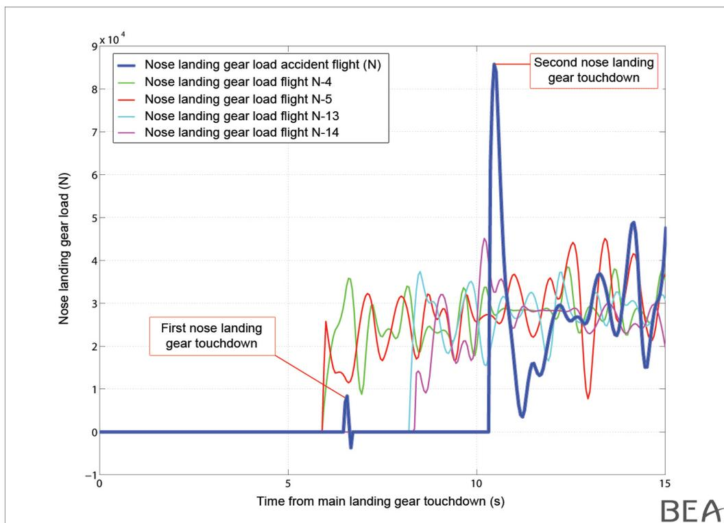
Figure 19: comparison of vertical loads on the nose gear
