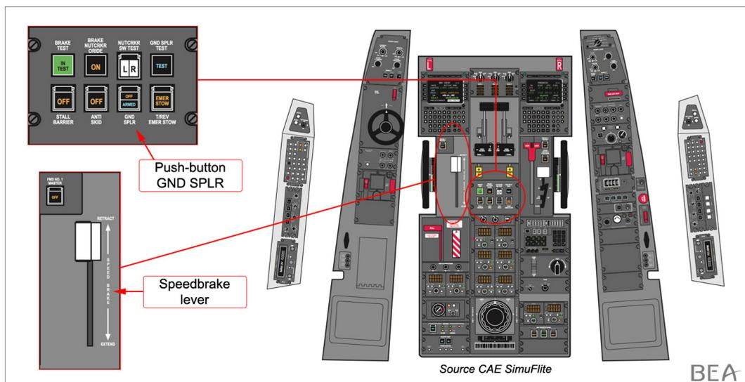
Figure 6: GND SPLR push-button and speedbrake control
